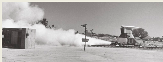
FIGURE 2.3.3 A rocket-powered sled used to test the effects of acceleration on humans.
